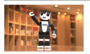
Sharp and NTT DATA SBC joined forces to develop an application that enables phone conversations for the hearing impaired by translating sign language to voice on Sharp's mobile Robophone. Robophone uses Deep Learning to recognize and analyze sign language movements, then speaks the words in Japanese to display the conversation on a smart phone, thus enabling communication.
